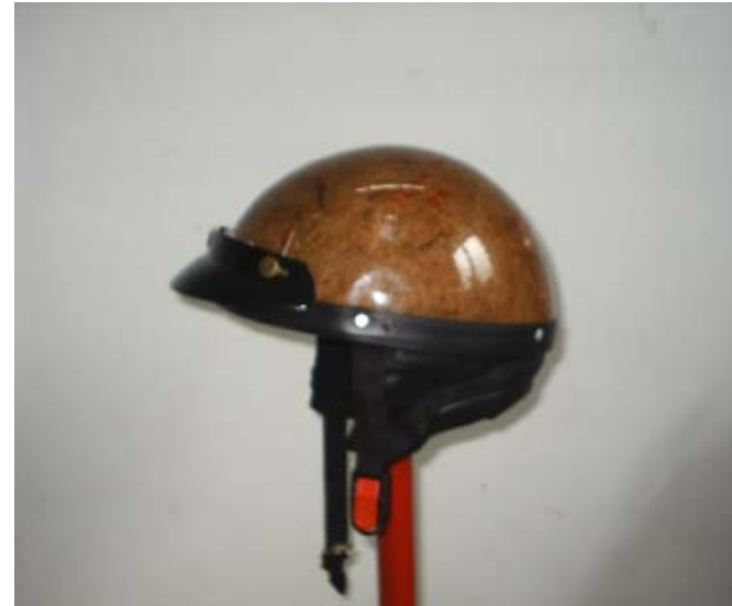
Helmet shell based on coconut fibre Faculty of Manufacturing Engineering, Universiti Teknikal Malaysia Melaka
